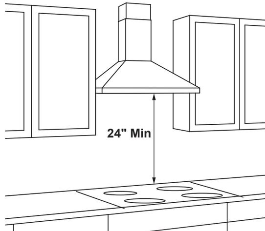
The vent hood must be installed 24" min. above the cooking surface. For optimal performance, installing the hood more than 38" above the cooking surface is not recommended. The hood installation height above the cooking surface depends upon ceiling height. The telescopic duct cover conceals the ductwork running from the top of the hood to the ceiling.
